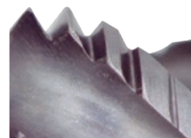
Close-up of VUSP after Tapping of 250 Holes
