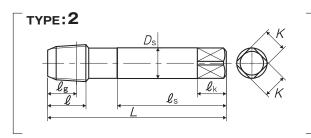
Segment: 1G Basic major dia (mm) ℓs (mm) Size Class Chamfer **MSRP** Code For Pipe Threads PT 1/16-28  ${\rm I\!I}$ SHX2T01K-8 2.5P 7.723 75 13.5 10.5 47 8 6 9 3 1 4,880 PT 1/8-28  ${\rm I\!I}$ SHX2T02K 2.5P 9.728 75 13.5 10.5 48 8 6 9 2 4,880 PT 1/4-19 SHX2T04-85 9 12 3 2 7,000  ${\rm I\!I}$ 2.5P 13.157 16.5 12.5 54 11 PT 3/8-19  ${\rm I\!I}$ SHX2T06-2.5P 16.662 95 18 14 60 14 11 14 3 2 ¥ 11,600 17 PT 1/2-14  ${\rm I\!I}$ SHX2T08Q 2.5P 20.955 105 22.5 17 64 18 14 4 ¥ 19,000
