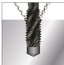
Chips from a tapped hole.
