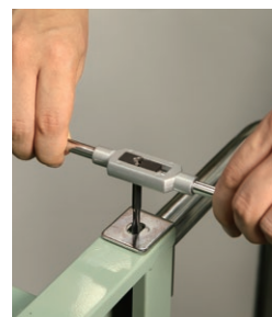
When hand tapping, always use tap wrench
