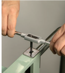
When hand tapping, always use tap wrench
