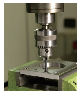
Machine tapping with drilling machine
