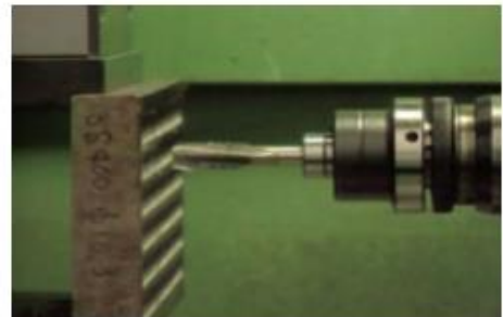
Chip configuration with the LO-SP tap
