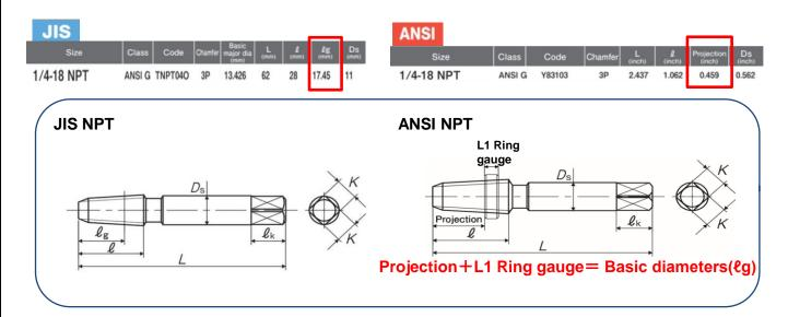
The "basic diameter position" for NPT (JIS) is calculated using the following method:
