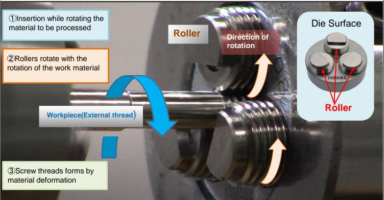
YAMAWA produces "DA SL", a die attachment for lathes that can easily attach rolling dies.
