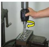
As shown in the photo above, the serial tap is similar in shape to a standard hand tap, but the height of the screw thread's crest increases in three steps, as illustrated in the left diagram.
