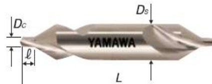
[Shape and dimensions in old JIS standard and YAMAWA standard]
