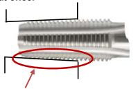
If the pilot hole is tapered, the tap starts cutting with it's entire outside diameter as it contacts the pilot hole. When contacting the pilot hole, the entire taper thread cuts into the workpiece at the same time. As a result, the taps thrust does not contact the cutting chamfer of the PT taps, so it can not be machined on asynchronous machines such as radial drilling machines. It will be necessary to process with a synchronous feed machine.
