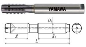
The HFICT-P and HFICT-B taps are cemented carbide that can tap cast irons at super high speeds. They are compatible with internal lubrication and by using a mist method to lower the temperature by a cool dry processing method. The HFICT-P utilizes side coolant ports for through hole tapping and it is suitable for cast iron. The HFICT-B utilizes a center through coolant hole shape and is suitable for blind hole tapping of cast iron.
