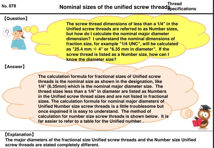
Fractional size Unified screw threads are calculated as  $1/4" = 1" \div 4 = .250$  in diameter or 25.4 mm  $\div 4"$  or 6.35 mm.
