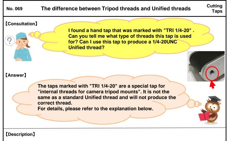
The "Hand Taps for Tripod threads HT TRI 1/4-20 " have the same thread form as the Unified threads, but the pitch diameter is approximately 0.2mm larger than that of the Unified threads.
