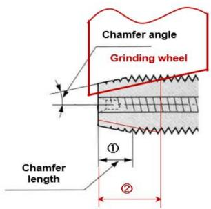
When taps are reground, it is essential to maintain the same chamfer angle to recreate an identical cutting performance to that of a new tap.
