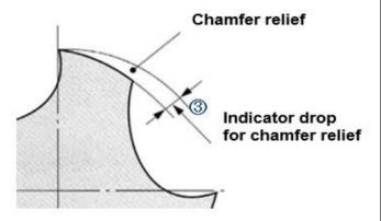
The chamfer relief is ground in a tangent curve to the outside diameter of the tap. The chamfer relief is not in a simple circular arc that is concentric to the diameter of the tap. The indicator drop for the chamfer relief ③ shown above changes depending on the tap type. It is difficult to select the indicator drop without proper instructions and reference
