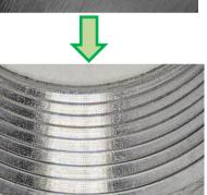
Tapping a tapered thread with a PT tap means cutting the internal thread to the correct length and thread depth with the threads on each flute of the tap. When the rotation of the tap is reversed, the thread tips of each land on each flute abruptly stop cutting the thread depth and the thread taper at the correct gage depth.
