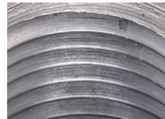
Smooth internal threads surface after being tapped by a SP-S-PT 1/4 tap.
