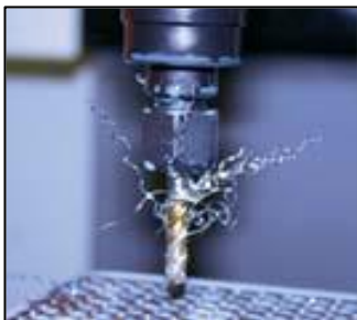
Drawing-1 Chip clogging in a spiral
