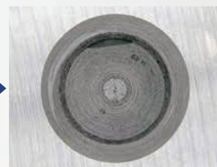
The remaining metal shavings inside the internal thread have been eliminated
