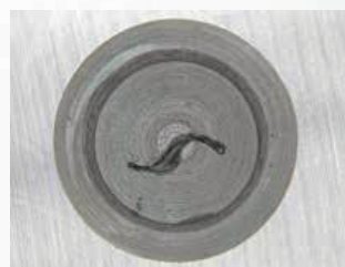
Drill bits and other debris remain
