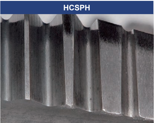
⚠ After tapping into 40 holes. Minimal wear and no chipping.
