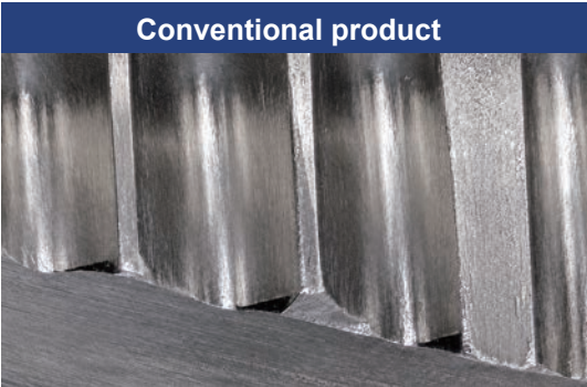
Chipping occurred after tapping 100 holes.
