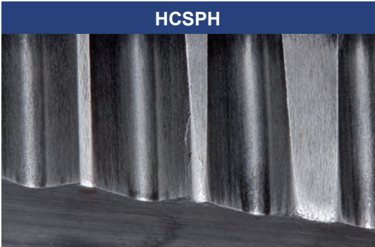
⚠ After tapping into 600 holes. Minimal wear and no chipping.
