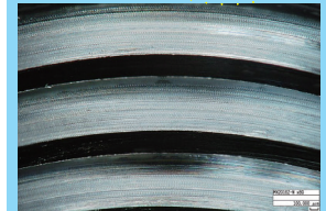
Left-hand spiral with surface treatment initial tapping Internal thread
