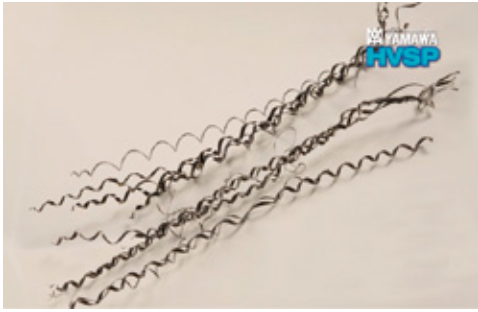
Ejected chips by large size taps
