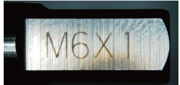
To keep a high accuracy of the shank diameter and circularity, the marking has been transferred from the shank to the square portion of the tap.
