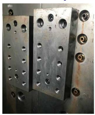
Several Rc (PT) screws are used for cooling holes.
