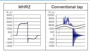
Consistent tapping in SCM440 (thermal refined) at 35HRC becomes possible. Before the MHRZ, this material was thought to be difficult for thread forming.
