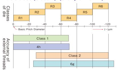
Class R shows PD tolerance of external screw thread formed by the rolling die.
