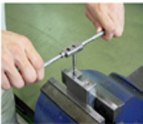
Manual tapping by using tap wrench
