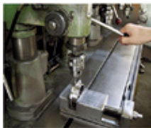
Tapping with drilling machine
